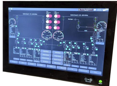
The LMA2101 offers access through displays of all sizes and the displays can be placed in any compartment of the vessel. The system can be extended with extra channels and the yard or the ship's crew can easily configure new alarms and create new layouts.
